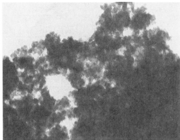
Figure 3. TEM micrograph of [1,4-(\text{H}_x\text{Si})_2\text{C}_6\text{H}_4]_n ; magnification 82 000.
